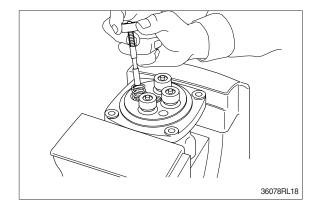
(3) Assemble O-ring (10) onto plug (8).
