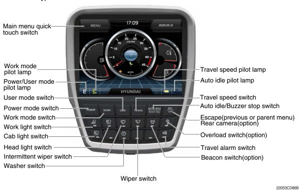
When some of the switches are selected, the pilot lamps are displayed on the LCD. Refer to the page 5-66 for details.
