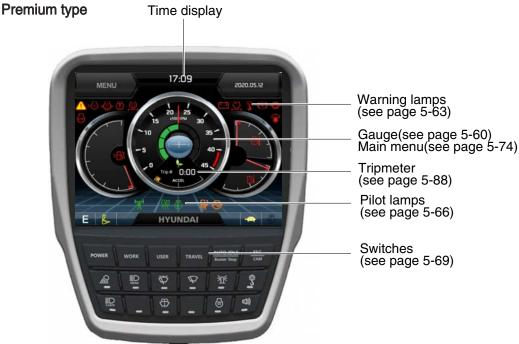
\* The warning lamp pops up and/or blinks and the buzzer sounds when the machine has a problem. The warning lamp blinks until the problem is cleared. Refer to page 5-63 for details.
