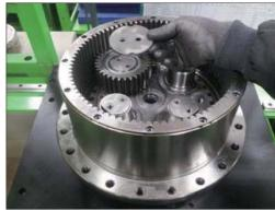
19) After spreading loctite #242, assemble the M10 bolt (64).(4 pcs)
