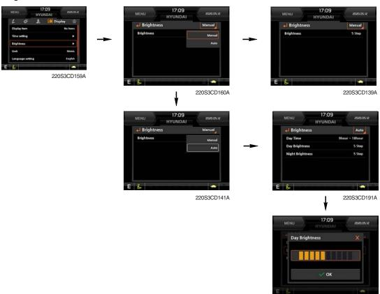
· If "Auto" is chosen, brightness for day and night can be set accordingly. Also by using the bar in lower side, users can define which an operation interval belongs to day and night. (in bar figure, white area represents night time while orange shows day time)
