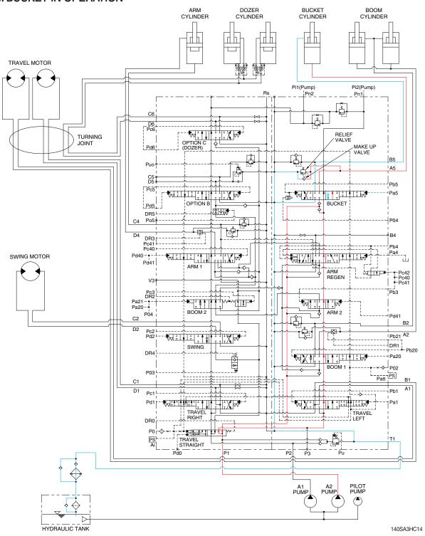
When the right control lever is pulled left, the bucket spool in the main control valve is moved to the roll in position by the pilot oil pressure (Pa5) from the remote control valve.
