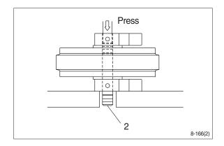
Remove the bushing (4) from idler, using a special tool. Only remove bushing if replacement is
