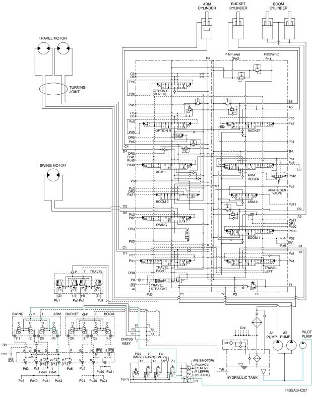
When the arm in control lever is tilted, the pilot oil from pilot pump flow into **Pc42** port in main control valve and the arm regeneration valve is shifted to left.
