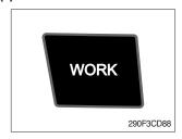
1 This switch is to select the machine work mode, which shifts from general operation mode to optional attachment operation mode.
