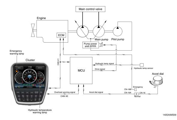
1. If the engine coolant temperature or the hydraulic oil temperature is overheated over set temperature, the warning lamp is ON and the pump input torque or the engine speed is reduced as below logic table.
