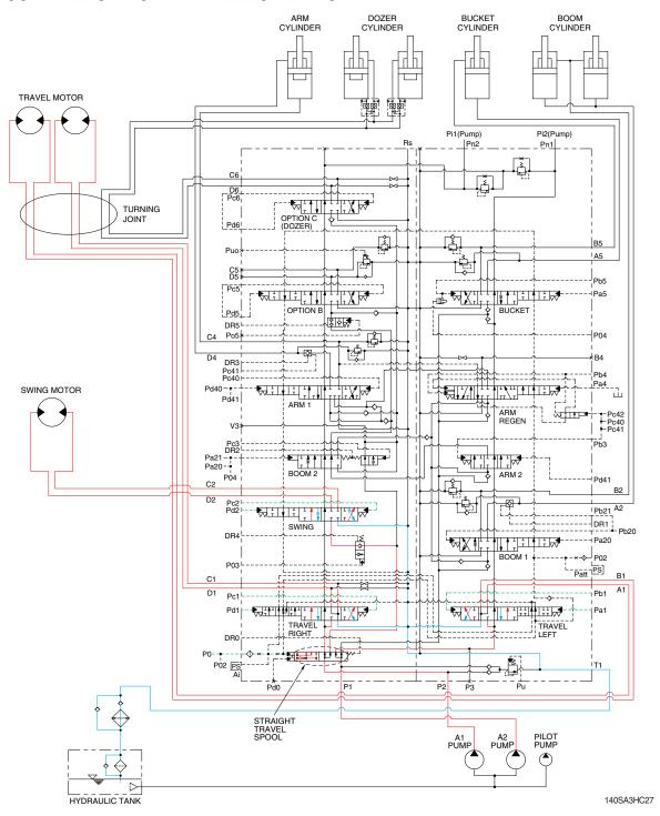
When the swing and travel functions are operated simultaneously, the swing spool and travel spools in the main control valve are moved to the functional position by the pilot oil pressure (Pc2, Pd2, Pa1, Pb1, Pc1, Pd1) from the remote control valve and straight travel spool is pushed to the right by the pilot oil pressure (P0, P01) from the pilot pump.
