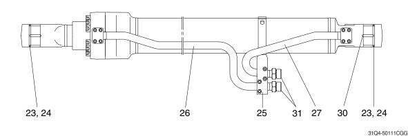
Tube assembly 12 Back up ring 23 Dimple bushing 1 2 Rod assembly 13 Cushion ring 24 Dust seal 3 14 Piston 25 Band assembly Gland 4 DD2 bushing 15 Piston seal 26 Pipe assembly-R 5 16 Wear ring 27 Pipe assembly-B Snap ring 6 Rod seal 17 Dust ring 28 O-ring 7 Back up ring 18 O-ring 29 Hexagon socket head bolt 8 Buffer ring 19 Back up ring 30 Socket plug 9 Dust wiper 20 Lock nut 31 O-ring 21 Hex socket headless set screw 10 Snap ring 22 Hexagon socket head bolt 11 O-ring
