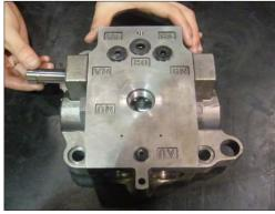
(18) Assemble plug (39-1) using hexagon wrench.
