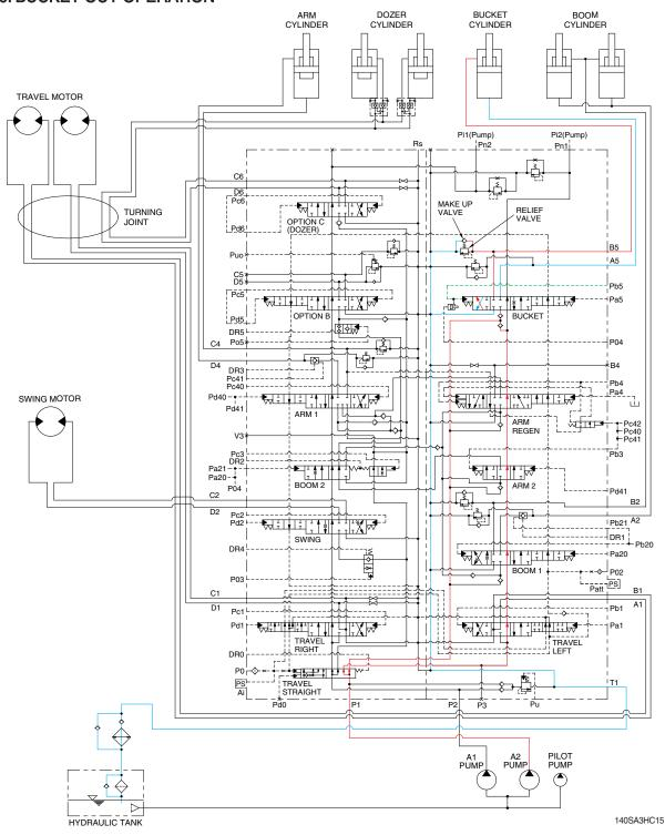
When the right control lever is pushed right, the bucket spool in the main control valve is moved to the bucket out position by the pilot oil pressure (Pb5) from the remote control valve.
