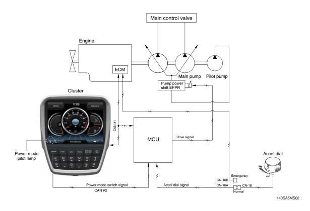
Mode selection system (micro computer based electro-hydraulic pump and engine mutual control system) optimizes the engine and pump performance.
