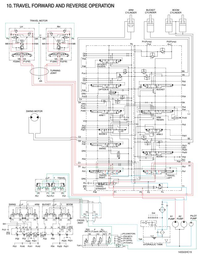
When the travel levers are pushed forward or reverse position, the travel spools in the main control valve are moved to the forward or reverse travel position by the pilot oil pressure (Pa1, Pb1, Pc1, Pd1) from the remote control valve.
