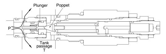
(4) The pressure at port P becomes lower than set pressure of the spring, the poppet is seated by spring force. Then the pressure at port P becomes equal to set pressure of the spring and the plunger is seated to the socket.
