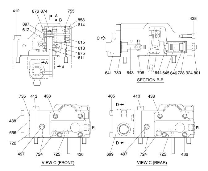
140SA2MP04 KR38-9NC2 (A1) KR38-9NC1 (A2) 079 735 722 466 Port Port name Port size P2 ⊦ Α Delivery port SAE 6000 psi 3/4" В SAE 2500 psi 2 1/2" Suction port Ρi Ρi Pilot port PF 1/4-15 Па 753 496 755 a SECTION D-D(REAR) Ρ1 В
