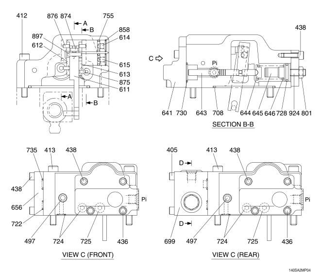
KR38-9NC2 (A1) KR38-9NC1 (A2) 079 735 722 466 Port Port name Port size P2⊦ SAE 6000 psi 3/4" Α Delivery port SAE 2500 psi 2 1/2" В Suction port PF 1/4-15 Ρi Pilot port Ρi 753 496 755 а SECTION D-D(REAR) P1 В
